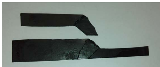
Figure 8. Tested tear specimen after 8 weeks of exposure to crude oil at 100 °C. [Color figure can be viewed in the online issue, which is available at wileyonlinelibrary.com .]
